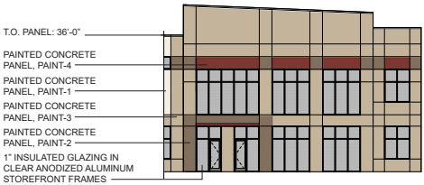
K-7 LOGISTICS CENTRE BUILDING 2 - ENLARGED ELEVATION (NOT TO SCALE)
