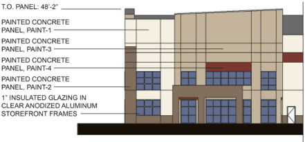
K7 LOGISTICS CENTRE BUILDING 2 - MATERIALS AND ELEVATIONS (NOT TO SCALE)
